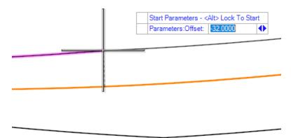
T. Snap to the intersection curve to set the end station.
