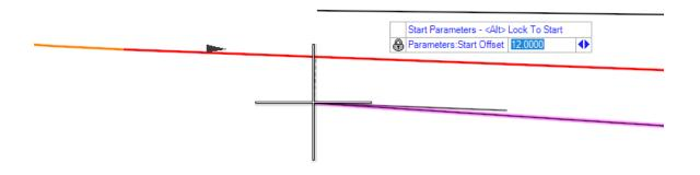
F. Move the cursor so the element moves towards the beginning of the alignment and left click to accept the offset of 12.00'
