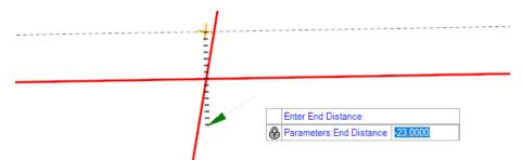
I. This will create the reference line perpendicular to Y8 located at the intersection of Y8 and Y18.
