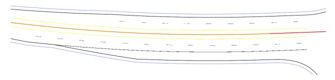
EE. Use the drag handles to adjust the start of the solid lane line to line up with the right lane bay taper.
