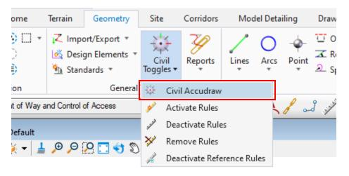
C. This will open the Civil Accudraw tool bar which can be docked by the Feature Definition toolbar.
