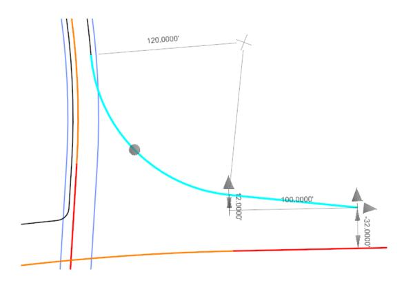
G. Now we have a right lane taper that ends tangent to the simple curve at a 12' offset.
