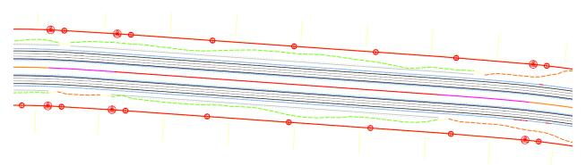
V. This completes the process of placing the RW lines and markers at a constant offset. The Default 3D model will show the 3D view of the marker placed at the correct elevation. These cells are the actual size of the marker and will appear small compared to some of the other elements.
