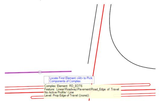
N. Left click to accept Back Offset of O'. Remember from the Horizontal tool training this is not the offset of the central curve but the offset of the tangent point from the reference element. The offset of the curve is handled by the specified taper offset.
