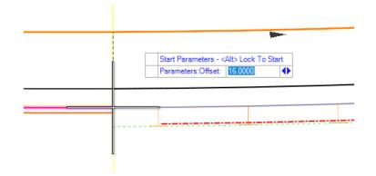
M. Use the <LEFT> arrow key to toggle to the length input and enter 22.875'. <ENTER> to lock and left click to accept.
