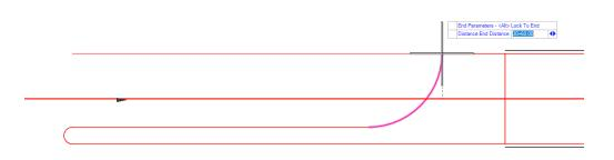
Y. We now need to create a 40' opening based on the standard. To do this we will shorten the line by 42', this will allow a nose with a 2' radius to be added while still maintaining the 40' opening. Start by using the **Element Selection** tool to highlight the element and activate the text manipulators.
