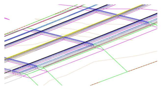
B. To add a vertical component to the guardrail elements we will get the elevations from the Y11 corridor. Start the **Profile From Surface** tool located in the *Vertical* section of the *Geometry* ribbon. This tool can add profile to multiple elements at the same time based on one or more surfaces, existing or proposed.
