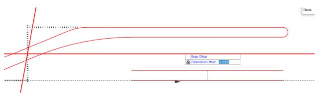
H. To create the nose of the island, use the **Simple Arc From Element** tool to create an arc with a 2' radius. Set the start point at the end of the inside island line.
