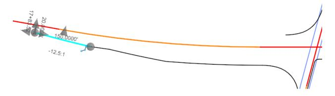
R. Using the same steps from above create a 300' taper to change the pavement width from 20' to 12'.
