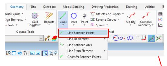
U. Draw a line connecting the sides of the approach slab.
