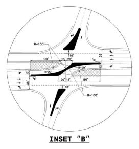
B. Begin with the island at the intersection on the left side of the road. Select the Single Offset Partial tool. Set the offset distance to 45.50' and offset the Y8 centerline to establish the edge of the island adjacent to the Y8 travel lanes.
