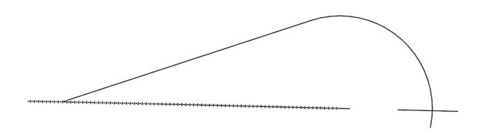
T. Use the **Trim to Intersection** tool from the same Modify group to extend the outside edge of travel line with the U Turn bulb at both ends. Select the edge of travel line not the Target Scratch 0 line.
