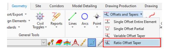
B. The dialog allows for the user to input the Begin offset and the ratio to the base element.
