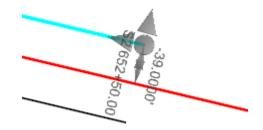
R. To construct the remaining portion of the edge of travel line that will be for the section with the 60' median select the **Single Offset Partial** tool. In this situation we can use the tool because we only want to offset a small portion of the L centerline, even though there will be no intervals.
