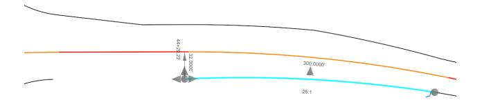
L. Using the **Single Offset Partial** tool now connect the lane drop taper to the intersection radius at Ramp C.
