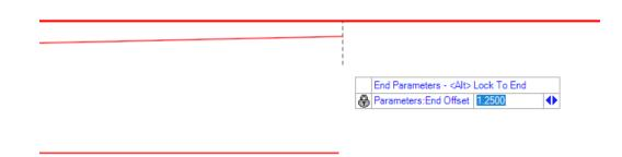
P. To set the end point location snap to the end of the previously constructed line. Because the offset is locked to 1.25' the offset will be maintained, but by snapping to the end of the previous line a rule will be created and any change to the length of the reference line will be reflected in the length, but not the offset, of the taper line.
