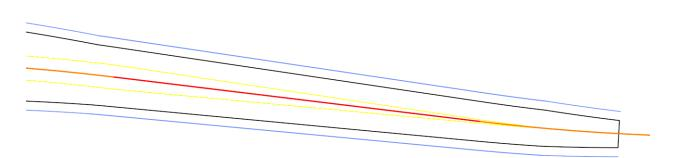
S. To create the skip lines for the thru lane, change the Active Feature Definition to TL PM White Dash
