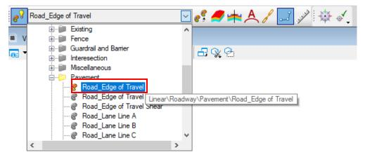
C. Select the **Single Offset Entire Element** tool. Use this tool because there will be very few breaks in the median pavement lines, only at bridges and overpasses.
