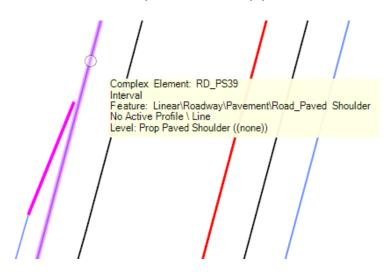
O. This will complete the paved shoulder transition from 6' on Y14 to 4' on Ramp A.
