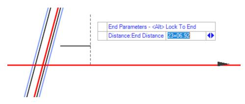
I. Left click near the bridge approach slab to set the end point. This location is not critical either, we will use the extend element tool to set the end point of the line.
