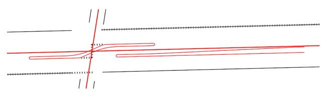
R. To create the center island at the U Turn Bulb we need to create a 40' opening at the U Turn Bulb.
