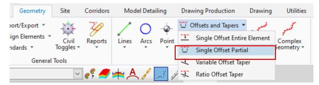
D. Left click to locate the reference element, use the left inside edge of travel. We will pick the inside edge of travel as the reference so that the rules are based on that element. If the inside edge of travel shifts for any reason the outside edge of travel will automatically adjust to maintain the 36' pavement width.
