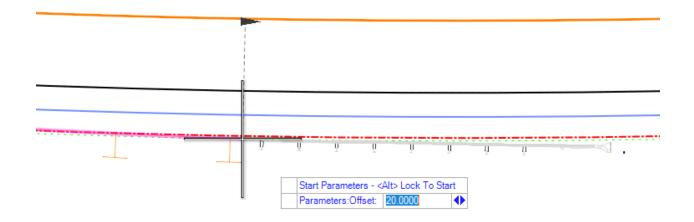
Y. Position the cursor so the end unit faces the correct direction and left click to accept the taper ratio of 50:1
