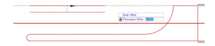
CC. To create the nose, use the **Simple Arc From Element** tool to create the island nose, this is the same process used previously, the radius is 2.00'.
