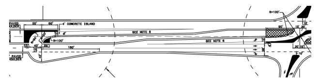
B. We will be adding the center turn lane island to the portion of the superstreet where the bulb is located on the left side of Y8.
