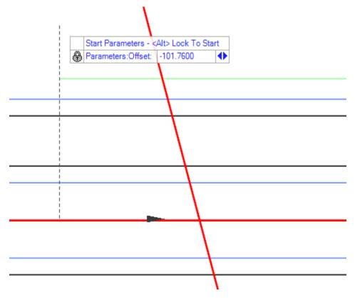
F. Left click to set a start point. The start point is not critical, we will use the modify tools later to complete the bridge, after offsetting for the bridge rail.
