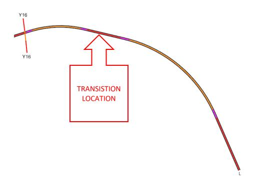
J. Use the **Element Selection** tool to highlight the left edge of travel line and activate the grab handles and text manipulators.
