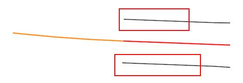
H. Turn on the FS reference file to display the existing edge of pavement. Using the Line **Between Points** tool draw a line from the end point of one element to the end point of the other. This is the begin pavement line.
