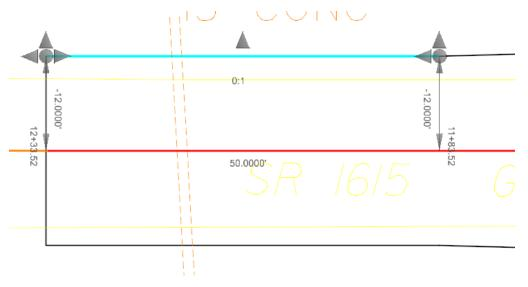
J. Select the drag handle arrow that is perpendicular to the centerline.
