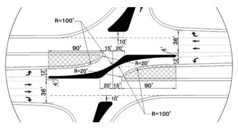
B. To start the process of laying out the island we will need a reference line to base all the offsets and measurements from. This line will be perpendicular to Y8 and located at the intersection of Y8 and Y18. This is the center point of the crossover median. Set the Active Feature Definition to Target Scratch 0
