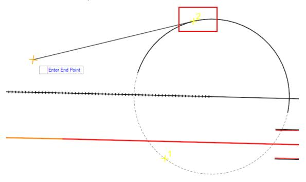
O. Snap to the end of the line that represents the end of the target line that represents the end of the taper.
