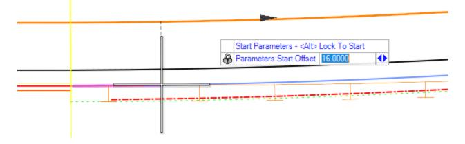
R. Place the cursor so the solution is line ahead and left click to accept the 50:1 taper.
