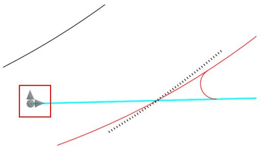
V. Use the drag handles to adjust the end of the reference elements to meet the 2' radius corner arc.
