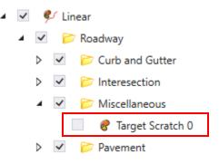
CCC. This will turn off the Feature Definition even though the level is still ON.
