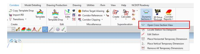
B. At the prompt locate the corridor by left clicking on the corridor. Note that the guardrail will only be visible in the dynamic section by selection the Corridor. If the centerline option is selected the guardrail and the guardrail flags will not be visible.
