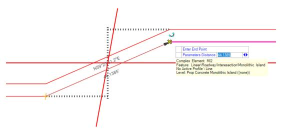
Q. The outside intersection point is known, it is based on the standard, and it has been marked using the reference elements. The inside intersection point will vary slightly based on the median width. This picture shows that the median width for the crossover portion is too narrow, it should be 4.0' minimum.
