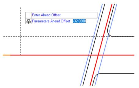
Q. Place the cursor in the outside quadrant to produce the correct result and left click to accept.
