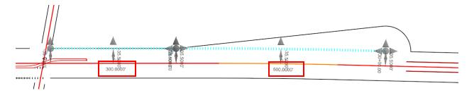
V. Note that the arc portion of the bulb stayed in the same place because the overall length is still 800'. The taper lengthened because there was a snap constrain created at the end of the Target Scratch line. The taper did maintain tangency to the arc because we used the Line to Element tool and the Trim Back option. By changing the Target Scratch Line length back to 180' the taper will update, and the arc will shift because of the snap constraint created when placing the arc.
