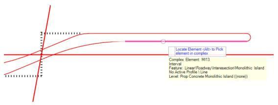
E. Offset this 17.50' to line up with the right outside of the crossover island. By using the **Offset Entire Element** tool, the end of the nose will automatically begin where the inside radius on the island starts. For different median widths and configurations, a different tool may be more appropriate.
