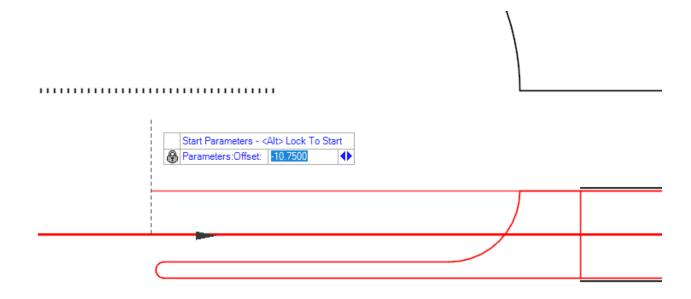
T. Snap to the end of the concrete island to set the start point and left click to accept.
