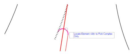
P. Snap to the end point of the arc to locate the start point.
