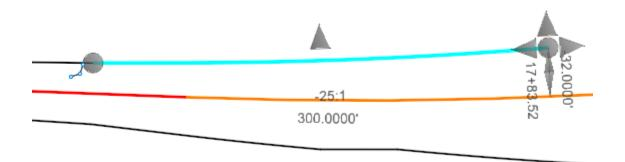
Q. The last step is to connect the edge of pavement taper line to the intersection radius at Ramp A. Using the Single Offset Partial tool, we will construct an element at a 32.00' offset.
