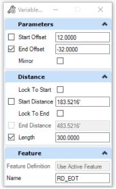
M. Select the Y14 centerline to start the tool. Snap to the end of the median taper, this will set the start station and offset for the lane drop taper.
