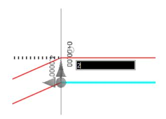
T. Repeat the process for the other side. The crossover portion will automatically update because of the snap rules that were created when placing the element using the Line Between Points tool.
