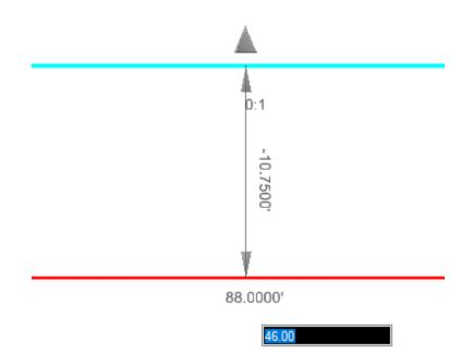
AA. This will shorten the line creating the desired gap. Note that using the text manipulator to change length the beginning of the line will remain in the same place and the length will change from the end. Because this line was place from right to left, the left end was the end that changed. This should be considered when placing the original offset element.
