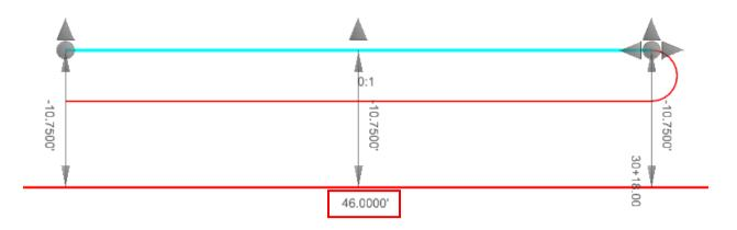
FF. Use the **Single Offset Partial** tool to create an element that is 10.75' offset and 254.00' long.
