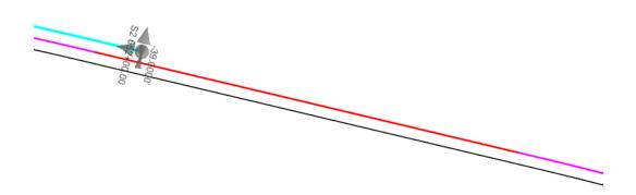
M. Use the **Element Selection** tool to select the right edge of pavement and highlight the drag handles and text manipulators.
