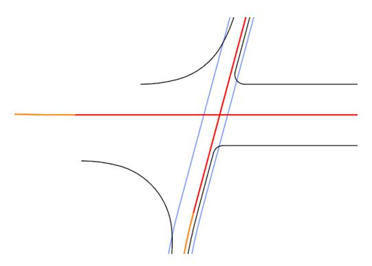
W. The Ramp C/D terminals are close enough to 90° that only a simple curve is required with a radius of 120'. The best tool to use is still the **Arc Between Elements** tool that was used for the 3 Centered Curves, this will allow for the offset to be specified and we can use the Y14 baseline as the reference element.
