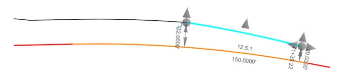
J. Use the Variable Offset Taper tool again to create a 300.00' median taper from an offset of 20.00' to an offset of 12.00'. We know we want this taper to match on the left and right side so set the mirror option to YES and create the right side automatically.
