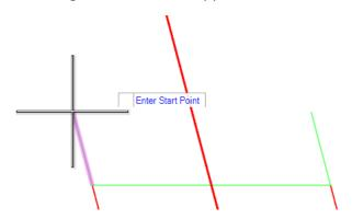
V. Snap to teach point to create a snap constraint. By doing that if the bridge length changes the approach slab will automatically adjust to maintain the design intent, which is a 25.00' long approach slab.
