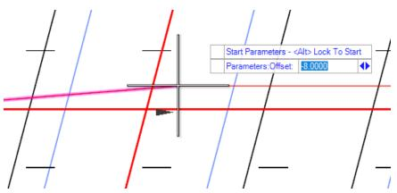
CC. To set the end station snap to the end of the radius at the Ramp D intersection.
