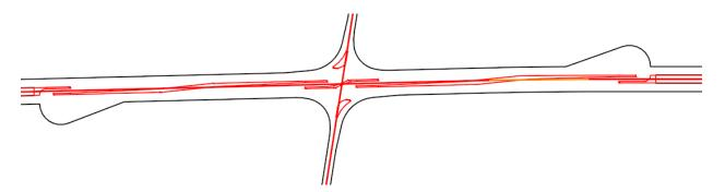
BB. To finish the design, create the outside 2'-6" curb and gutter line. Set the Active Feature Definition to Road\_Curb and Gutter 2ft-6in.
