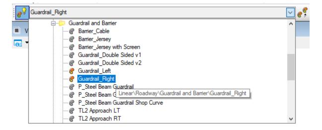
K. Using the **Single Offset Partial** tool create a guardrail element parallel to the Y11 centerline that starts at the end of the bridge rail and is 22.875' long. This represents the B-77 Structure Anchor Unit. Left click to select the Y11 centerline.
