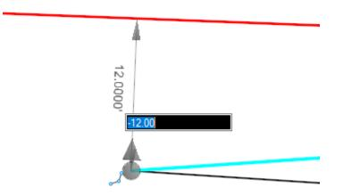
K. This will correct the offset and create a taper that matches the taper on the right side.
