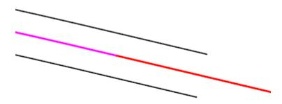
Q. Use the **Element Selection** too to pick the left edge of travel and activate the drag handles and text manipulators. Change the station to 652+50. Note that the right edge of travel lines automatically adjusts to the same station. This is because of the snap rule created in the previous operation.
