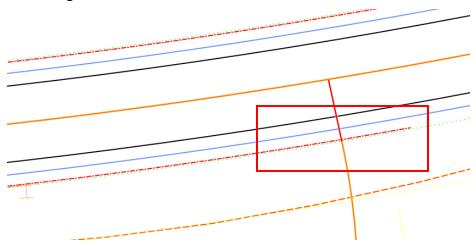
U. Add a Type TL-3 Anchor unit to the end of the previously placed guardrail and terminate the guardrail prior to the Y9 intersection. The Anchor Units are also line styles, but they will have the appearance of a cell. Set the Active Feature definition to TL3 Trail RT. It is important to use the correct feature definitions, the line styles used with ruled geometry and that have 3D components cannot be "flipped" around as easily as they could in SS2.
