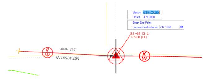
L. To place a RW line on the right side type in S2 624+00 and offset of 195.00' and <ENTER> to lock the station and offset.
