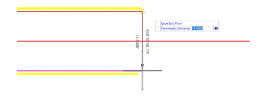
F. To add the corner radius on the island, select the **Simple Arc** tool from the **Arc Between Elements** tool group.
