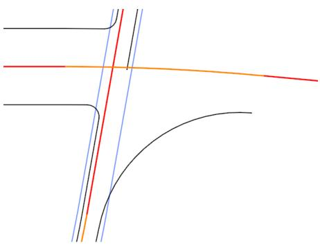
EE. Repeat the process with the same setting for the Ramp D terminal except for the offset, which should be changed to 44' to allow for a right turn lane.
