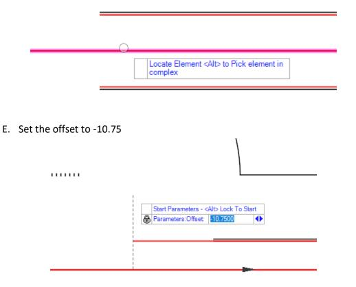
F. Left click to the end of the Arc portion of the U Turn bulb to set the start point.
