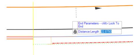
N. Set the mirror option to NO and left click to accept, this will create the structure anchor unit parallel to the centerline.
