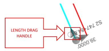
O. Drag the line back to the end of the left edge of travel line. Snap to the left edge of travel line to set the end of the right edge of travel line. This will also create a snap constraint.
