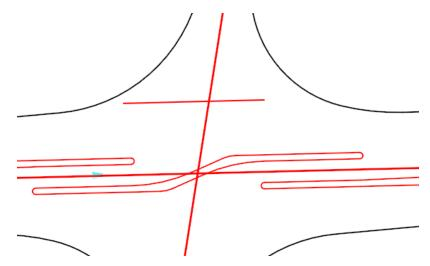
D. To construct the right side of the island, use the **Single Offset Partial** tool and construct an element offset 2' from the Y18 centerline.
